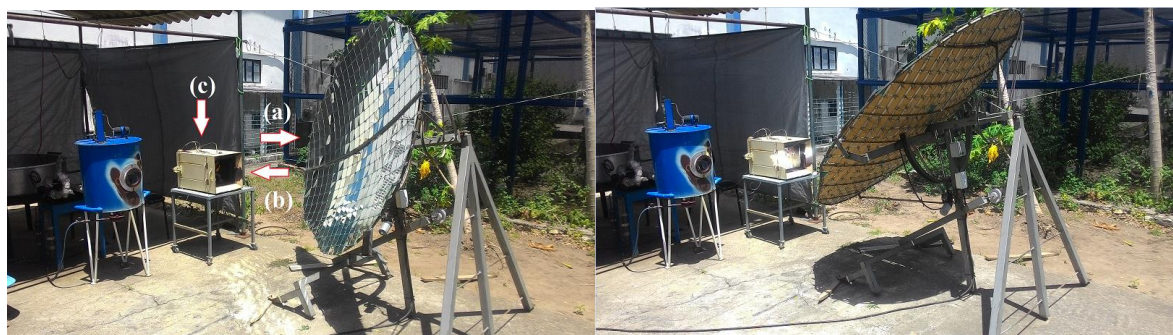
(a) concentrador solar, (b) forno solar e (c) termopares.
